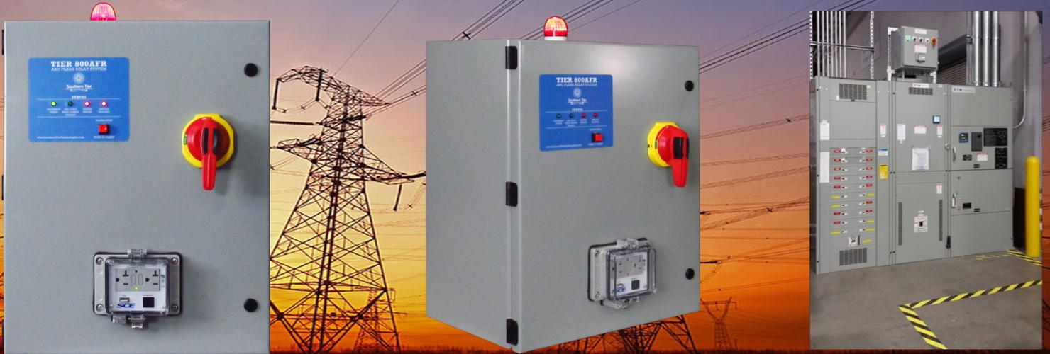
The Tier 800AF Series Arc Flash Relay System reduces arc flash incident energy and boundaries in both Medium-Voltage and Low-Voltage electrical systems. The Tier AF series is an externally installed control cabinet that uses up to four fiber optic sensors to immediately detect light associated with an arc flash event and quickly activate a system disconnect.
